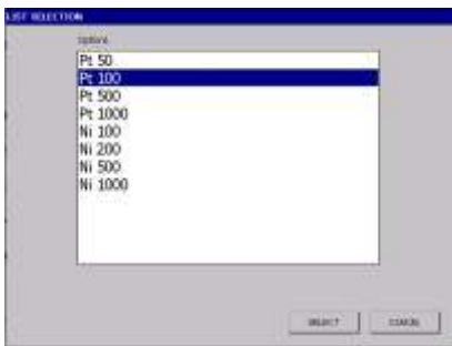
Figure 6.23 Linearization Select (Input Type Resistance Thermometer)
